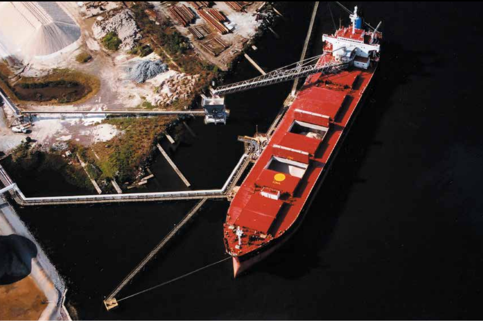
Unloading aggregate into a hopper.
